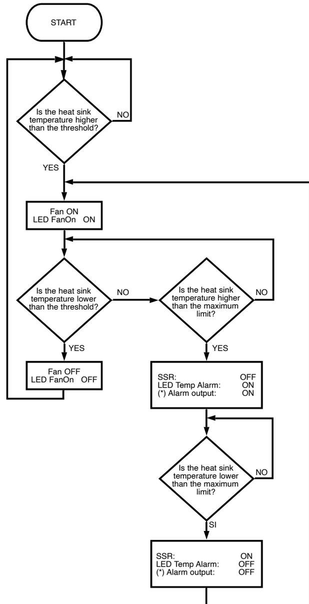
(\*) Turned on alarm output only in case of versions with on-board diagnostic options (D-1/2/3 and A-2) on pins 14 and 15.
