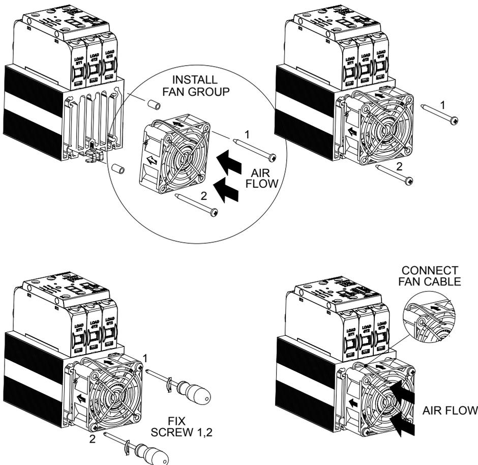
Use a Phillips screwdriver with a max. diameter of 3.5mm.
