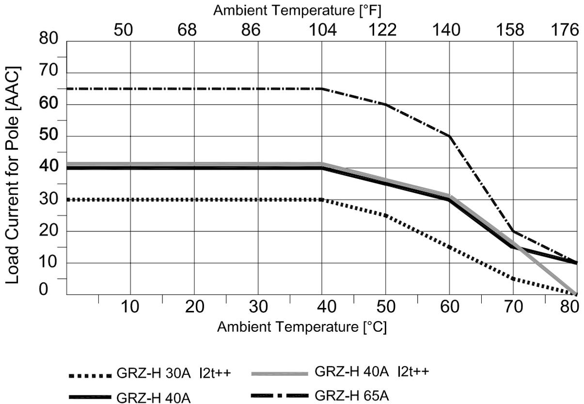
Note: The curves of the GRZ-H 40A/ 65A refer to the device complete with a working standard fan.
