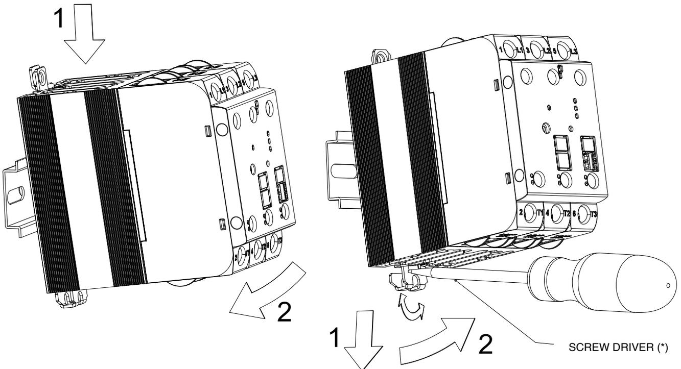
(\*) Use of a slotted screwdriver with a max. diameter of 6mm is recommended
