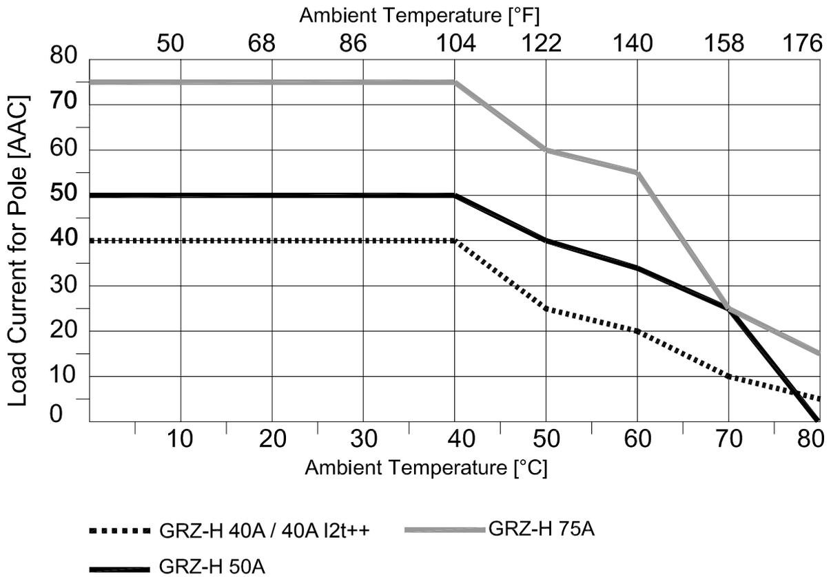
Note: The curves of the GRZ-H 50A/75A refer to the device complete with a working specified fan.
