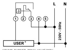
\* PUMP, BURNER. ZONAL VALVE WITH SPRING RETURN.
